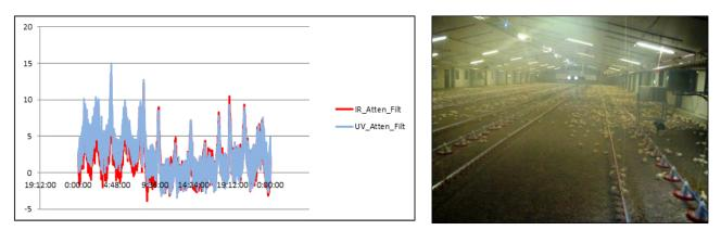
The example below is from a site where water mist is sprayed every few minutes, 24/7 to maintain a humid environment. In a trial using OSID (Imager 10°) over a distance of ca. 40-50m, no water droplets or condensation occurred on the Imager or Emitter lenses. The graph below shows a 30 min period. There is little differentiation between UV and IR, hence the site operated without false alarm or faults.
