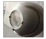
Water condensing on an Imager or Emitter is the result of their surfaces' temperature cooling below the dewpoint of the air which is in contact with them.
