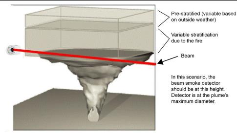
Since it is difficult to predict the resulting stratification depth, it may prove necessary to install multiple layers of detectors at lower heights. Because the plume is narrower nearer the base of a fire than at the stratification or ceiling level, supplementary beam detection will also have to be installed closer together. Refer to section 3.4 for spacing information.
