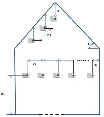
For the earliest detection of a rising smoke plume within a high open space area, the width of the area protected on each side of an optical beam is 12.5 % of the height of the beam above the highest likely seat of a fire.
