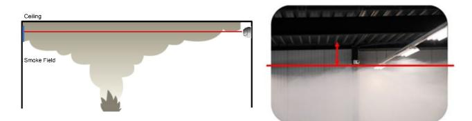
The depth of stratification under the ceiling can vary significantly between summer and winter as well as through the effect of the developing fire itself.
