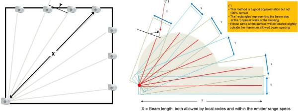
Y = Beam coverage, width allowed by local codes and with
