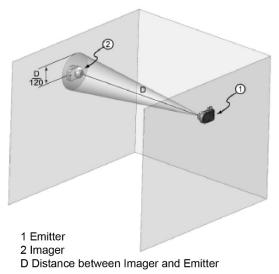
Given the danger of accidently commissioning the wrong Emitter due to a poorly aligned Imager, the system installation must meet the following conditions for this new mechanism to work.
